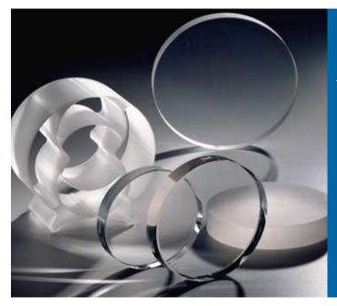
HPFS<sup>®</sup> Standard Grade, Corning code 7980, is a high purity synthetic amorphous silicon dioxide manufactured by flame deposition. The noncrystalline, colorless, silica glass combines a very low thermal expansion coefficient with excellent optical qualities and exceptional transmittance in the ultraviolet. It is available in a number of grades for different applications.
