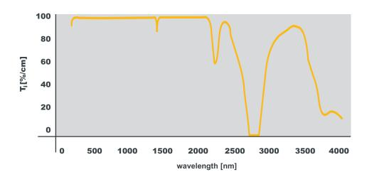
HPFS<sup>®</sup> Standard Grade is certified to meet T external ≥ 80%/cm @185nm (T internal ≥ 88%/cm @185nm), when measured through a polished, uncoated sample.
